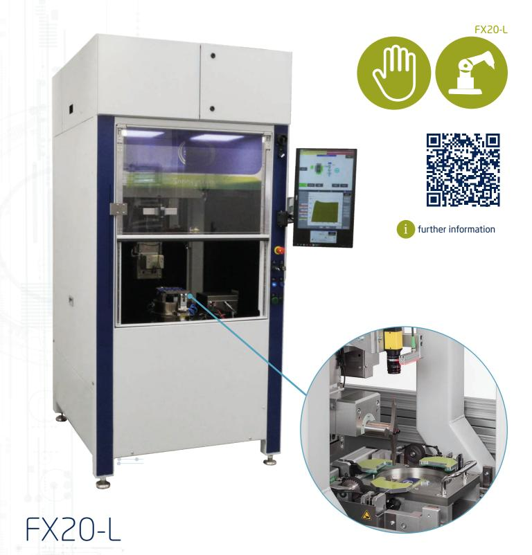
The FX20-L is a semi-automated ultrasonic welding machine for production. It is suitable for welding power electronic modules (e.g. IGBT modules) or cell contacting systems (battery applications). The machine is available with a pattern recognition system for checking and correcting the welding position and an external particle cleaning system.
