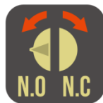
Color Match / Mismatch Output Mode Switch
